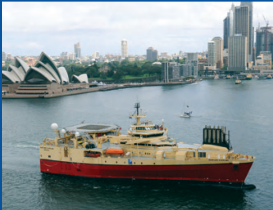
Ramform Sterling is the newest vessel in the PGS fleet, capable of towing up to 22 streamers.
