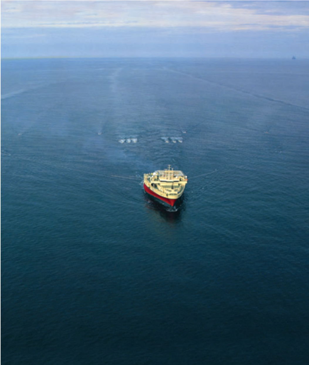
The delta-shaped hull with an extremely wide aft beam is characteristic of the Ramform design, here Ramform Valiant is carrying out seismic acquisition.
