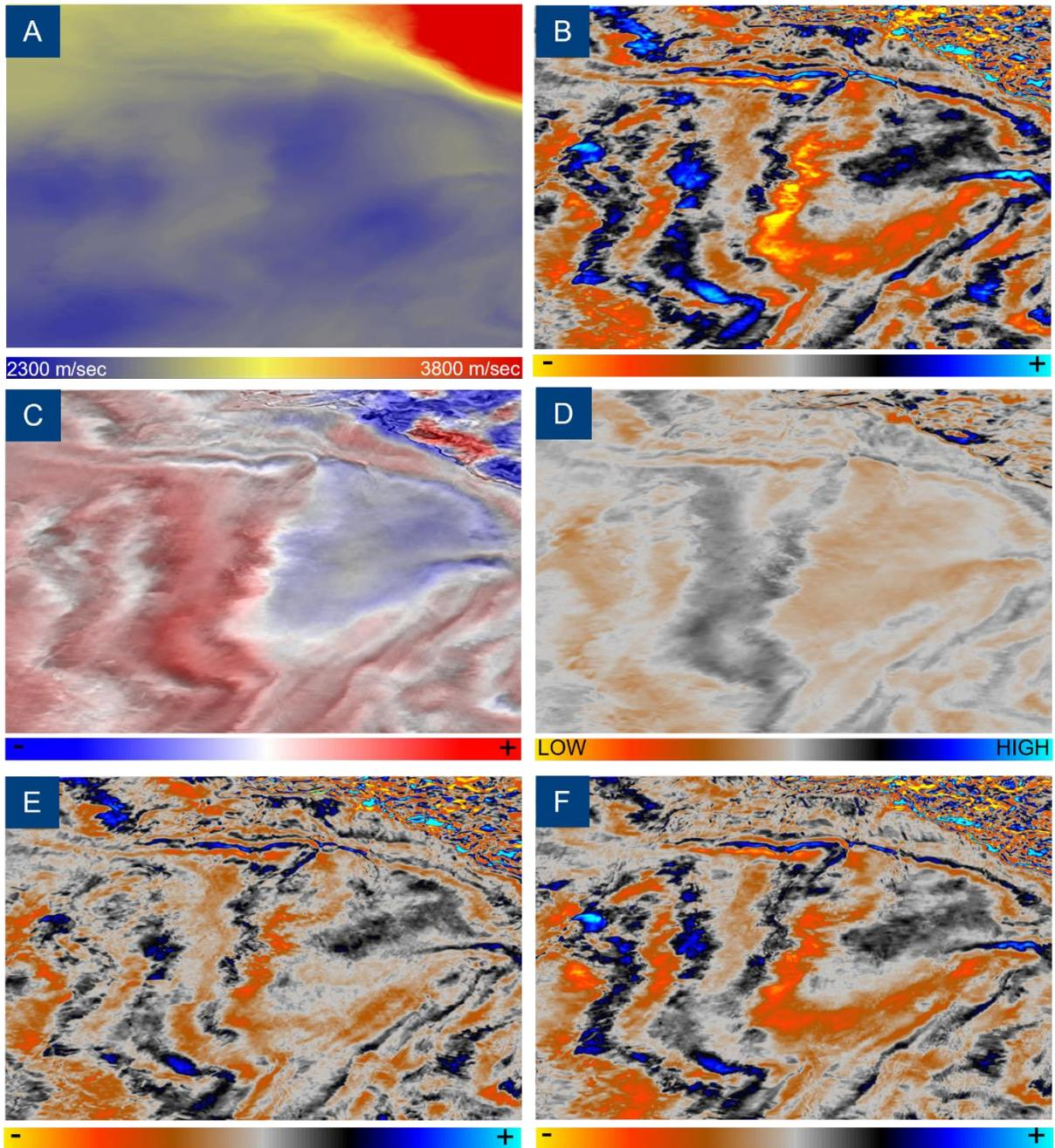
**Figure 3:** Depth slices extracted at reservoir level (5000m) for: (A) inverted velocity, (B) full-stack reflectivity, (C) velocity perturbation overlaying structural image, (D) relative density, (E) near-stack reflectivity, and (F) far-stack reflectivity.
