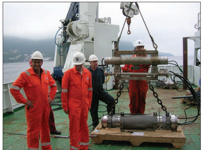
Figure 3: A 2-gun Bolt Annular Port Gun cluster hanging from a gun frame, with the near-field hydrophone and pressure transducer mounted.
