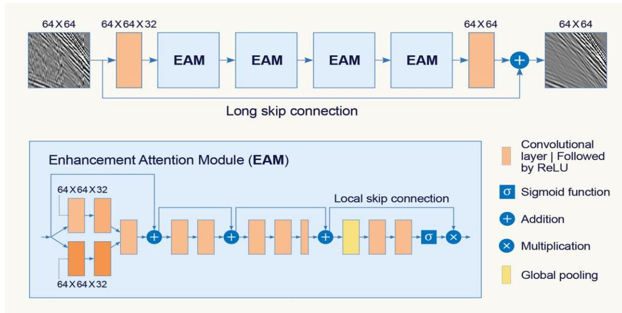
**Figure 1** Schematic of the RIDNet convolutional neural network architecture.
