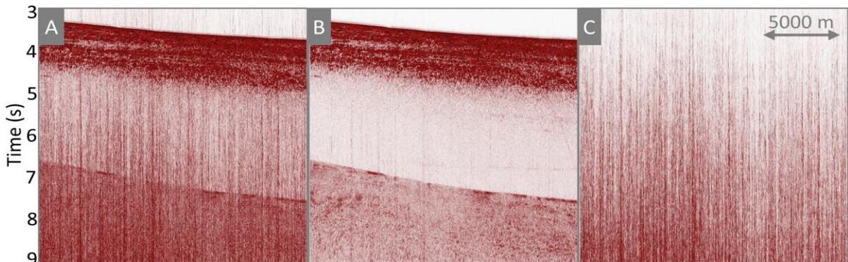
**Figure 5** 2D QC stack of particle motion records a) before and b) after the noise attenuation. c) noise attenuated by the workflow. A 20-30 Hz Ormsby lowcut filter was applied to the input to the stacks.
