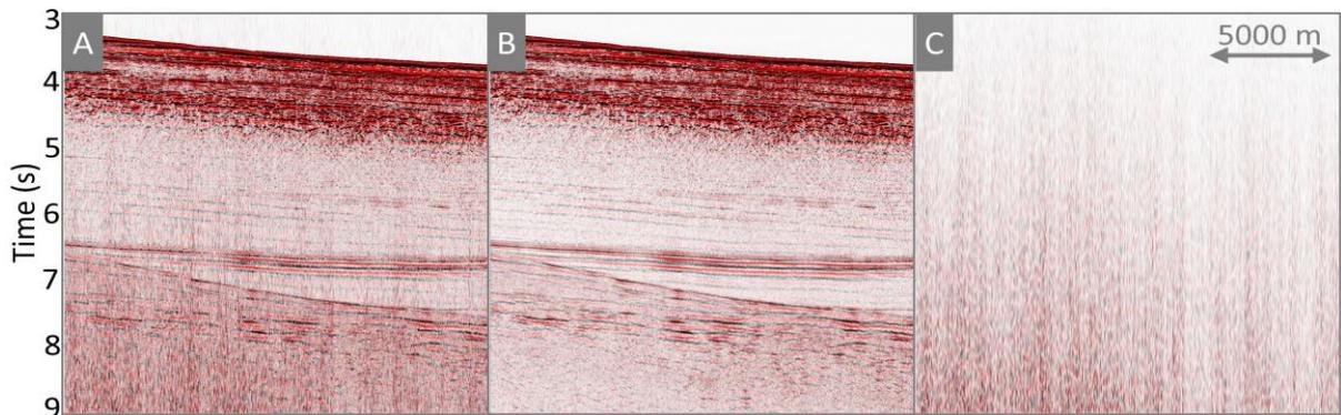
**Figure 3** 2D QC stack of pressure records a) before and b) after the noise attenuation. c) noise attenuated by the workflow.
