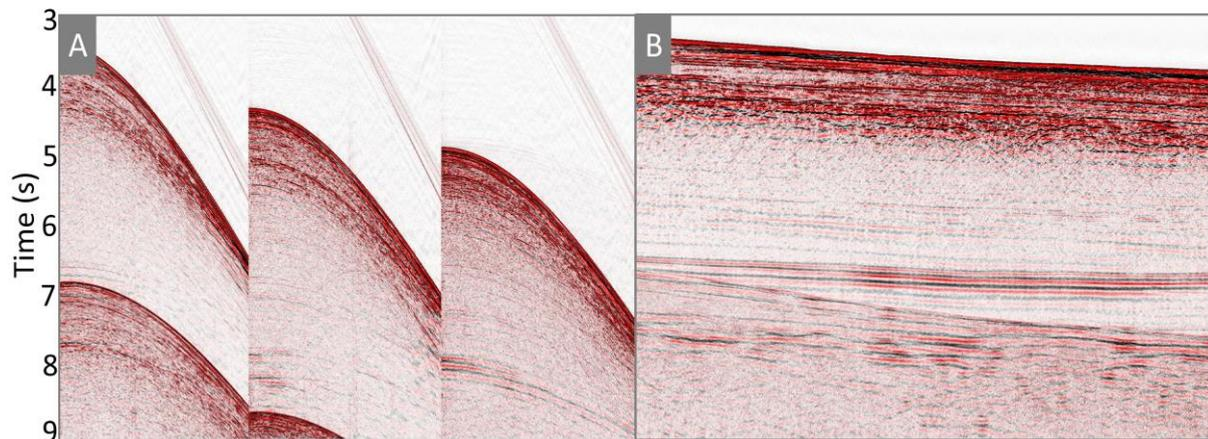
**Figure 6** Shot gather examples (a) and 2D QC stack (b) of the up-going pressure field generated from the noise attenuated pressure and particle motion records.
