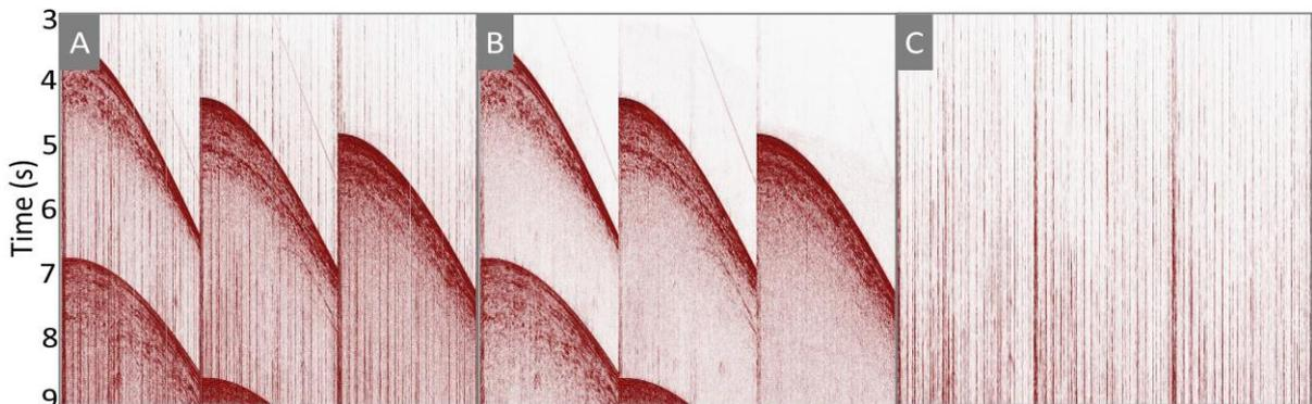
**Figure 4** Shot gather examples of particle motion records a) before and b) after the noise attenuation. c) noise attenuated by the workflow. A 20-30 Hz Ormsby lowcut filter was applied for display purposes.
