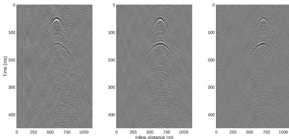
**Figure 5** Three adjacent common receiver gathers with 1.5625 m trace spacing within each gather.
