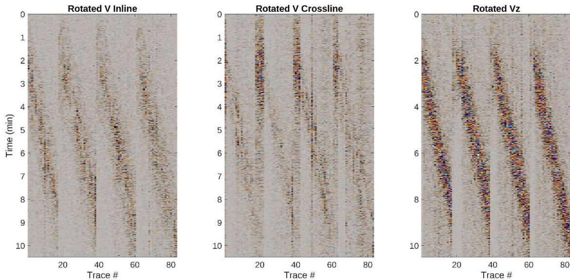
**Figure 2** Three component geophone measurements from four adjacent ocean bottom cables with a 50-100Hz band-pass filter after vector rotation such that the original vertical component is pointing in the direction towards the vessel as a function of time (right panel).
