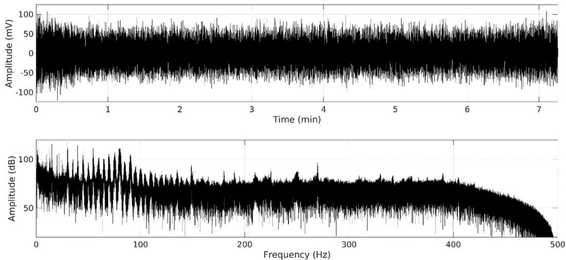
**Figure 4** Time series of the estimated wavefield generated by the vessel emitted in the vertical direction (top), and the amplitude spectrum of this time series (bottom).
