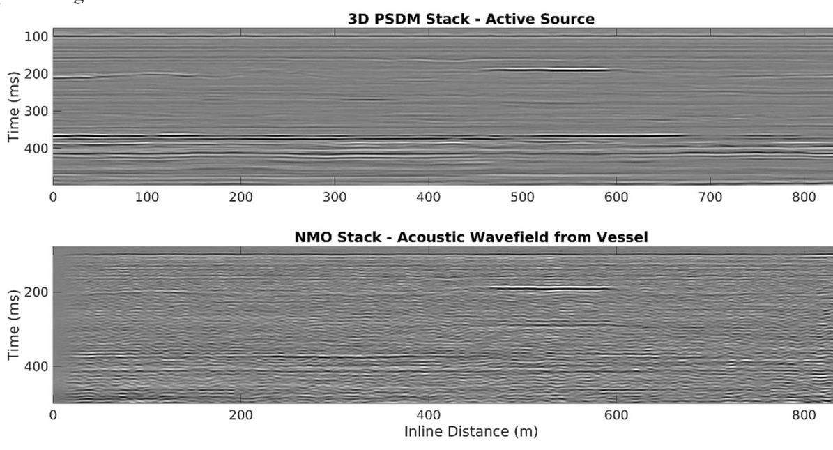
**Figure 6** The line along the vessel path from the 3D PSDM stack volume acquired with airguns (top), and the NMO stack of the data using the acoustic wavefield generated by the vessel as a source (bottom).
