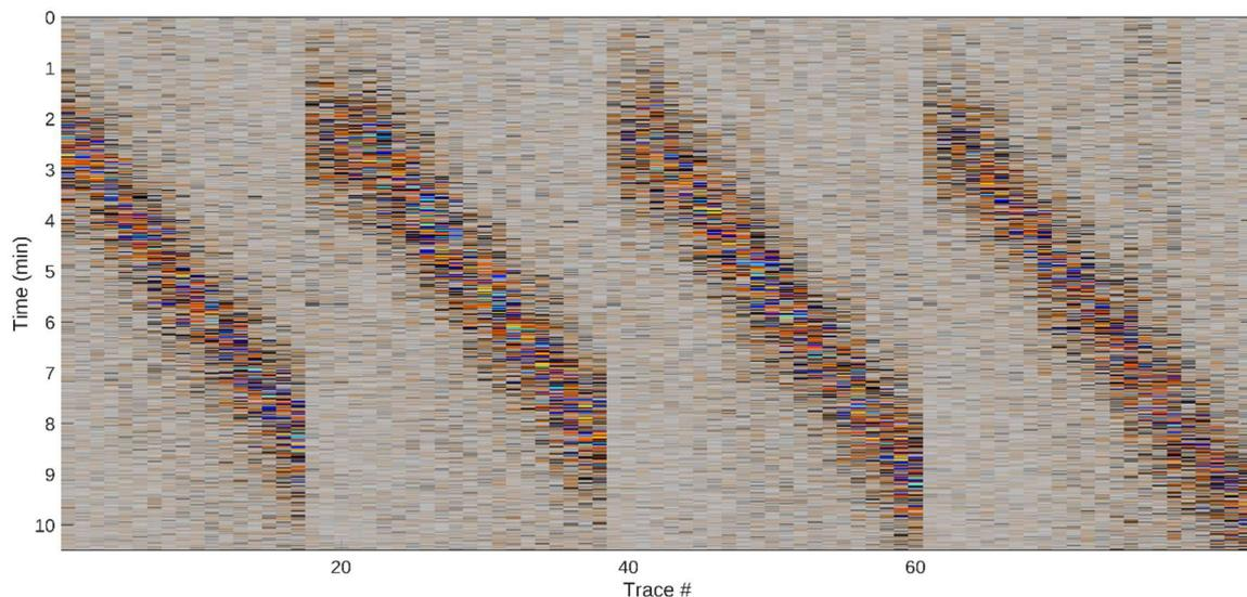
**Figure 1** Recorded hydrophone data from four adjacent ocean bottom cables with a 50-100 Hz band-pass filter to highlight the signals coming from the vessel.
