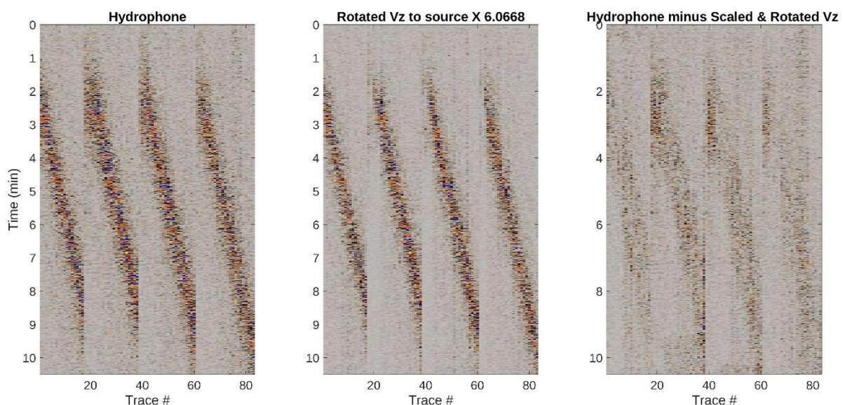
**Figure 3** Hydrophone data (left), scaled and rotated geophone data pointing in the direction towards the vessel (middle), and the difference between these (right).
