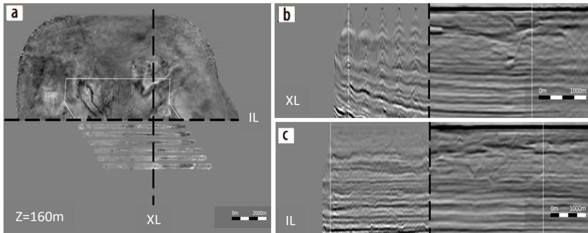
**Figure 3** Images from separated wavefield imaging (3a top; 3b/c right) and primaries-only WEM (3a bottom; 3b/c left). Slice at 160 m depth, and crossline and inline up to 400 m depth. The image from separated wavefields has improved illumination in the shallow, and images between and well beyond the cable patch.
