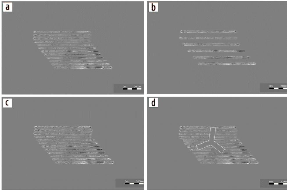
**Figure 4** Decimation tests results: Primaries-only WEM imaging at a depth of 160 m for (a) no decimation, (b) decimation to every 2<sup>nd</sup> cable, (c) decimation to every 4<sup>th</sup> receiver on a cable, (d) platform hole decimation, outlined by the white polygon.
