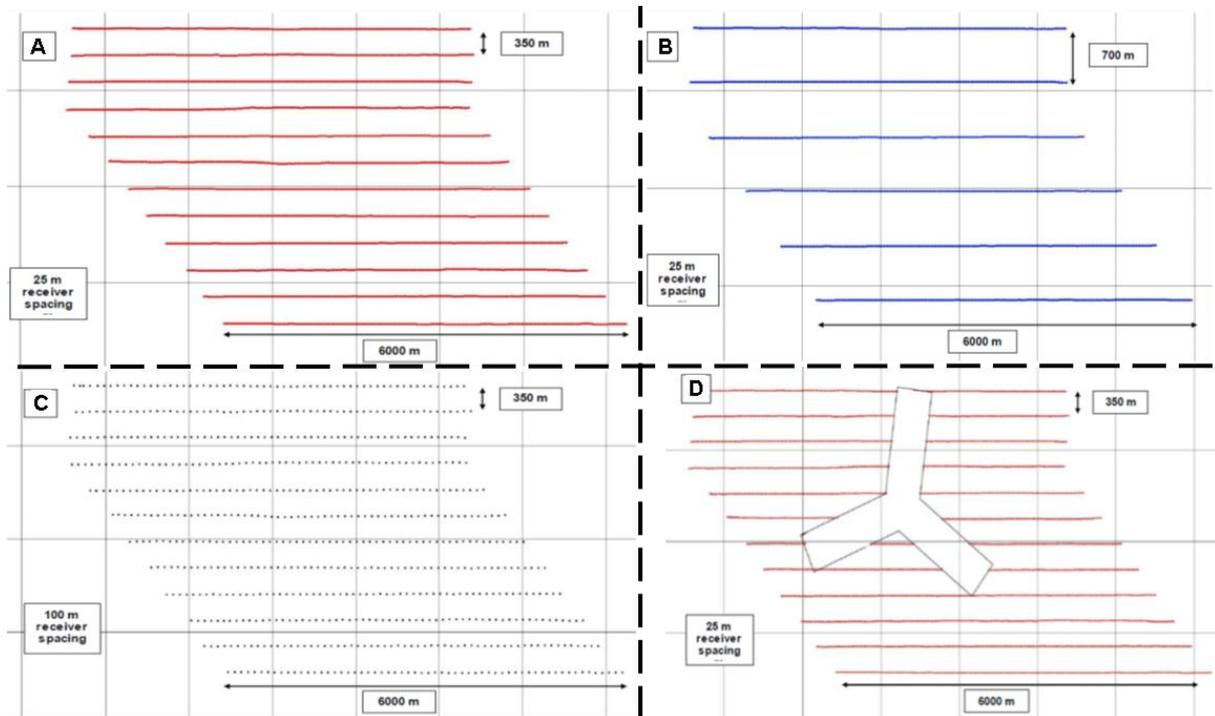
**Figure 2** Decimation tests: top view of ocean bottom cable layout for (A) no decimation, (B) decimation to every 2<sup>nd</sup> cable, (C) decimation to every 4<sup>th</sup> receiver on a cable, (D) platform hole decimation.
