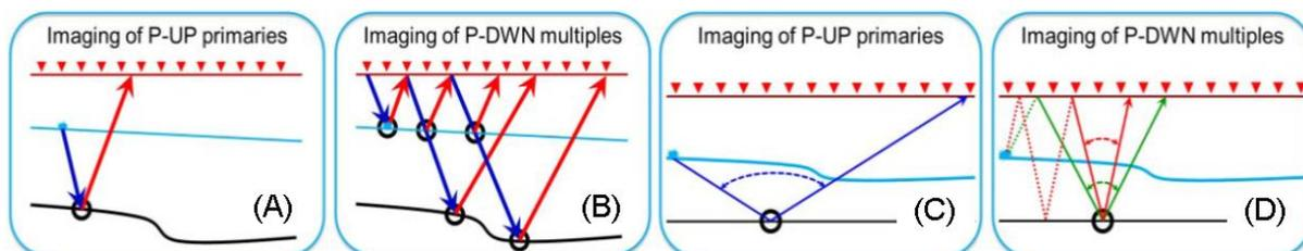
**Figure 1** Sketch of ray-paths used in OBS imaging, after applying reciprocity: (A) imaging of primaries using up-going wavefield (P-UP); (B) imaging of multiples using down-going wavefield (P-DWN). Blue and red arrows denote source and receiver wavefields, respectively. Imaging locations are indicated with circles. (C) Reflection angle from primaries using up-going wavefield; (D) reflection angles from multiples using down-going wavefield.
