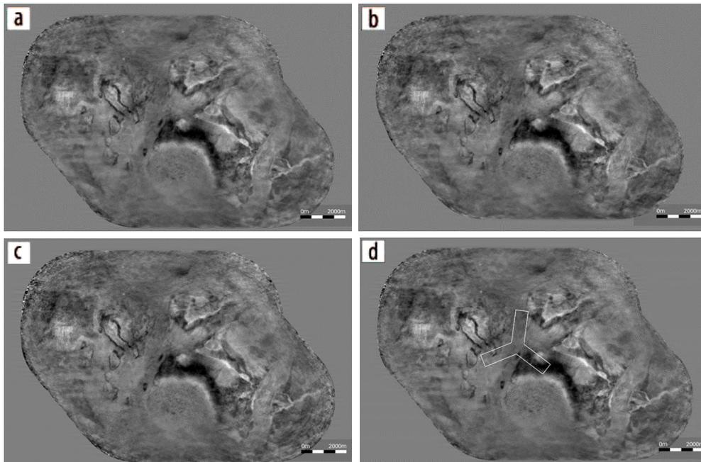
**Figure 5** Decimation tests results: Separated wavefield imaging at a depth of 160 m for (a) no decimation, (b) decimation to every 2<sup>nd</sup> cable, (c) decimation to every 4<sup>th</sup> receiver on a cable, (d) platform hole decimation, outlined by the white polygon. Note images (a) to (d) look almost identical; separated wavefield imaging is not adversely affected by decimation in this test.
