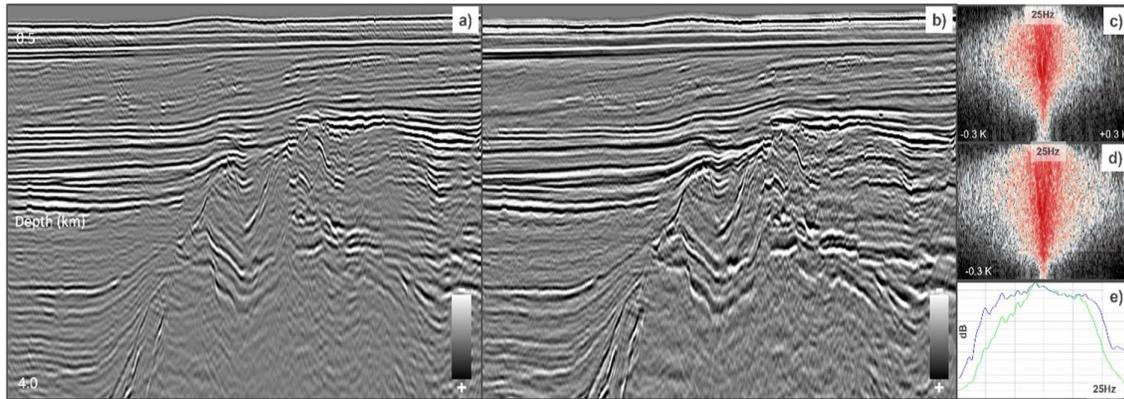
**Figure 1** Comparison of RTM (a) and the new data-domain LS-RTM (b) with the corresponding FK-spectra in (c) and (d). Comparison of the amplitude spectra are shown in (e), where the green curve corresponds to RTM and the blue curve shows the LS-RTM. Notice the improvements in the wavenumber content, amplitude fidelity, structural imaging and fault mapping in the LSRTM results compared to the RTM.
