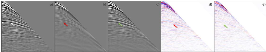
**Figure 3** Recorded shot gather after full pre-processing (a), synthetic data with the initial reflectivity/velocity models (b) and with updated models (c) and the corresponding initial (d) and updated data-residuals (e). Notice the improved data-match after inversion and the reduction in the data-residuals after inversion, as annotated by the arrows.
