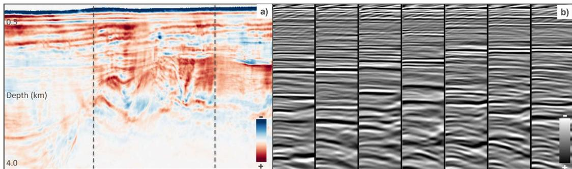
**Figure 2** Accumulated velocity difference with  $\pm 100$  m/s display range (a) and imaging QC of the refined velocity model through the centre of the line, between the two stipulated lines (b). The velocity updates are structurally consistent with the image and produce flat angle gathers computed with wave-equation migration.
