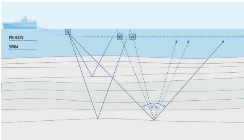
**Figure 2** Separated Wavefield Imaging (SWIM) uses sea-surface reflections recorded by dual-sensor streamers to recover near-angle information even in very shallow settings with Source (S) and Virtual Source (VS).
