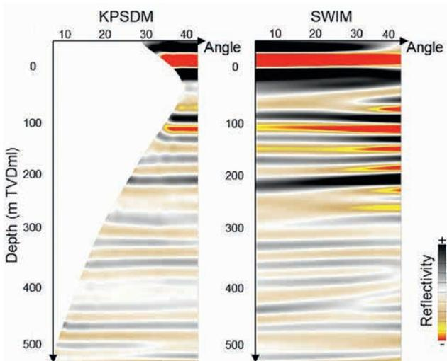
**Figure 3** At the Jurassic target 250 m below the seabed K-PSDM (using primaries) delivers minimum recorded angles of 24 degrees whereas SWIM delivers near-angle traces down to 3 degrees by using sea-surface reflections.
