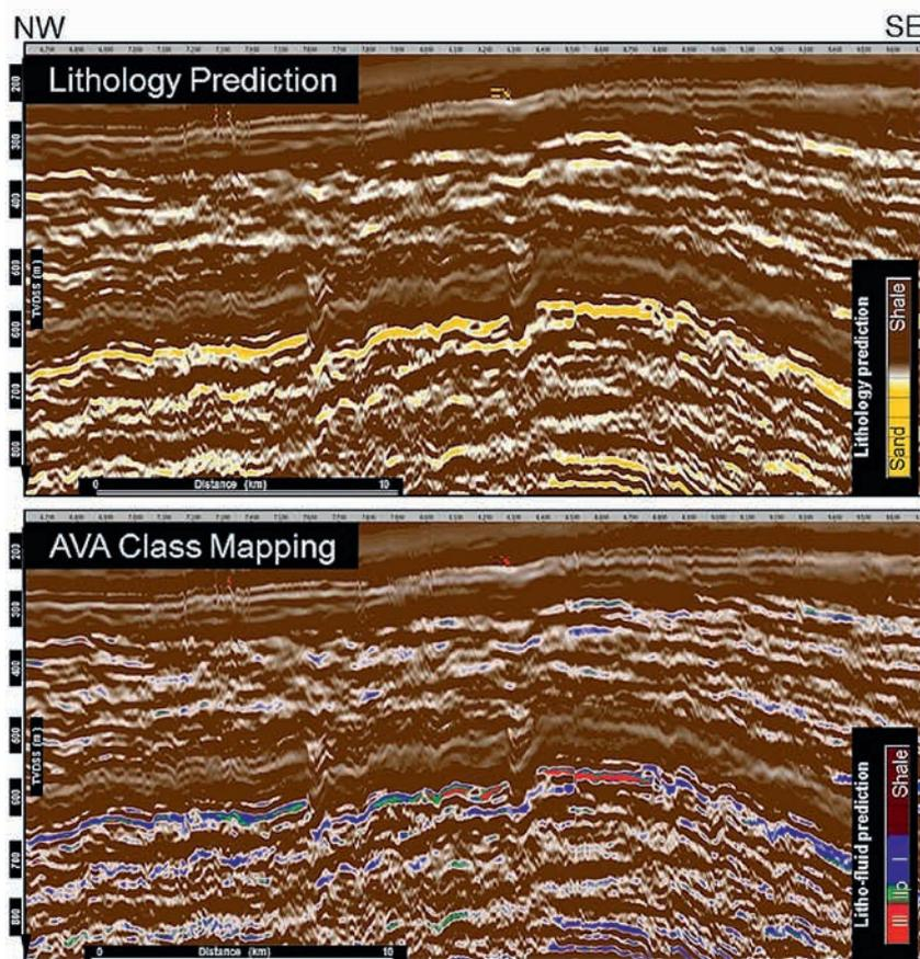
Figure 12 Lithology classification and AVA class mapping using AVA rotations in the relative  $I_p$  versus relative  $V_p/V_s$  domain.
