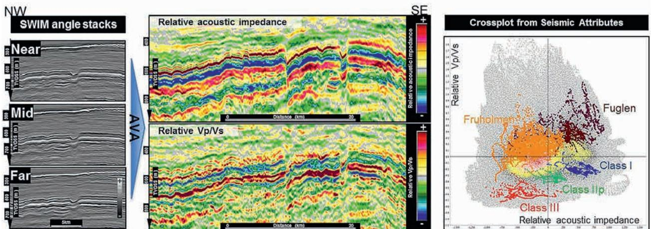
**Figure 11** Relative  $I_p$  and relative  $V_p/V_s$  estimation using separated wavefield imaging pre-stack information leading to lithology and AVA class detection.
