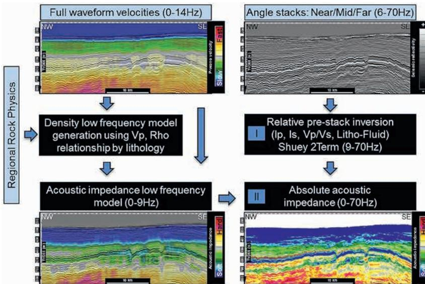
**Figure 10** Quantitative interpretation workflows integrating separated wavefield seismic data and FWI P-velocities for reservoir characterization in areas with limited access to well information.
