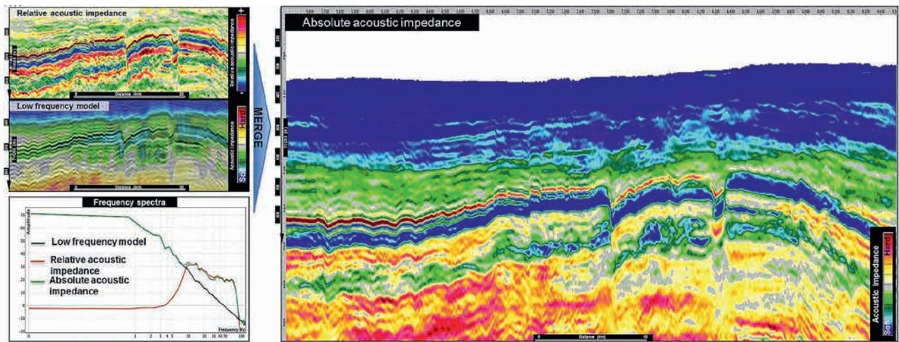
**Figure 13** Absolute acoustic impedance obtained by merging scaled relative acoustic impedance with an acoustic impedance low frequency model derived from FWI.
