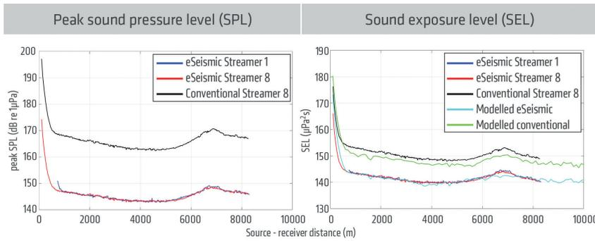
**Figure 6** Peak sound pressure levels (SPL) to the left, and sound exposure levels (SEL) to the right.
