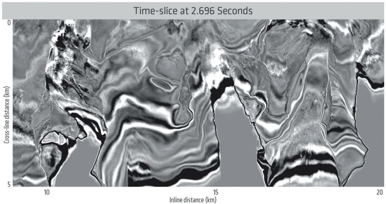
**Figure 8** A time-slice from preliminary migrated results of the field trial survey demonstrating high signal-to-noise levels and the ability of the proposed novel acquisition method to resolve fault boundaries in great detail, aided by the significant increase in spatial source sampling.
