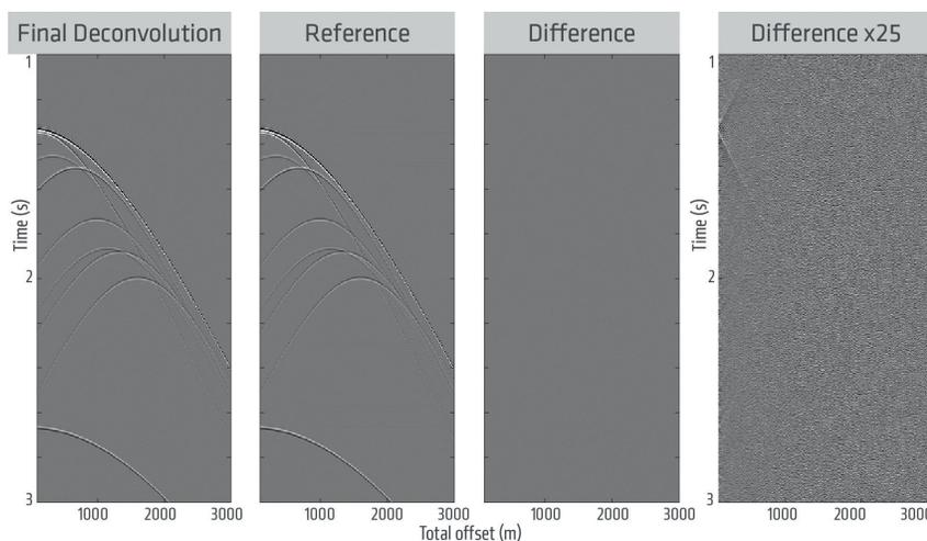
**Figure 3** Final deconvolution result of a continuous synthetic receiver trace in a stationary location (first panel to the left), the desired result (second panel from the left), the difference between the actual result and the desired result (third panel from the left), and finally the difference multiplied by a factor 25 (fourth panel from the left).
