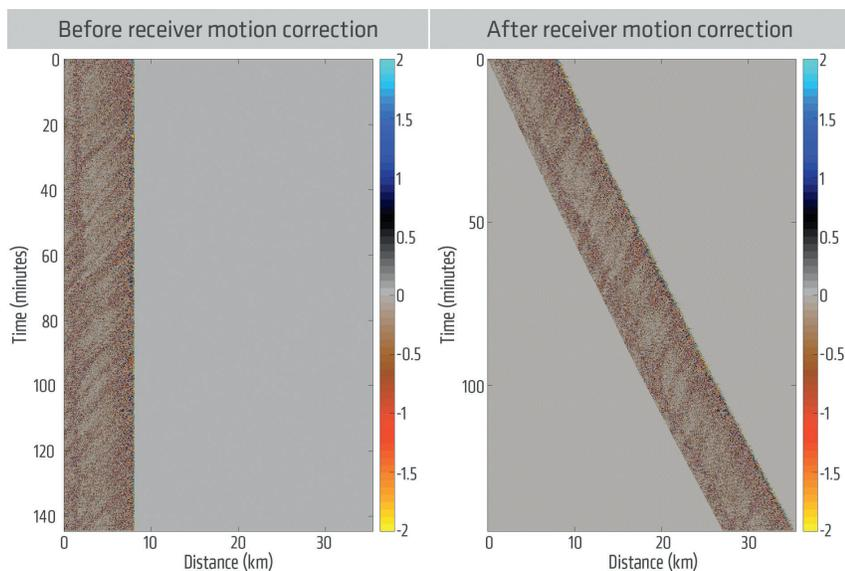
**Figure 2** One continuous seismic record from one sail line before and after correcting for the receiver motion. Each data trace after receiver motion correction represents one stationary receiver location.
