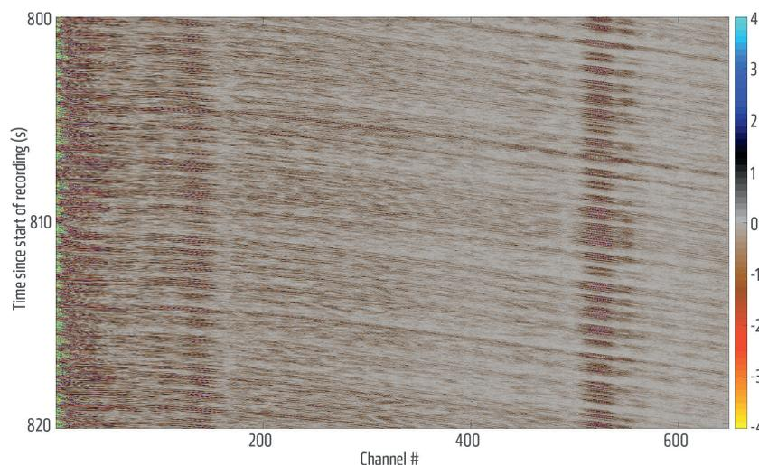
**Figure 1** A 20-second portion of a continuous seismic record with raw hydrophone data, with signals generated by triggering individual air guns with short randomized time intervals.
