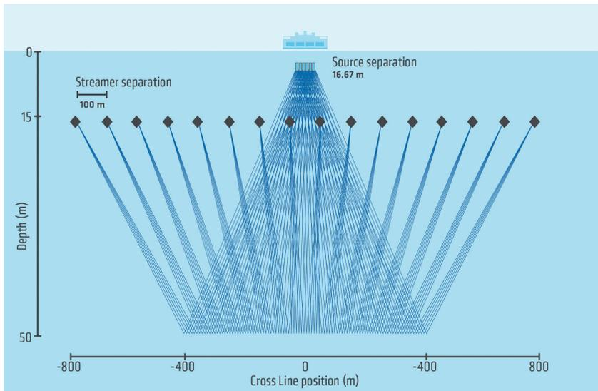
**Figure 4** Illustration of the acquisition configuration cross-line used for the 3D test survey.
