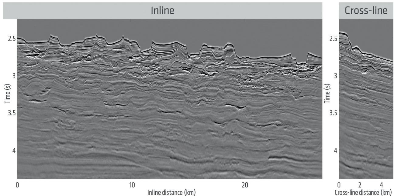
**Figure 7** An in-line and a cross-line from preliminary migrated results of the field trial. Data shows high structural detail, especially in the shallow part of the section and great lateral resolution across the whole of the section.
