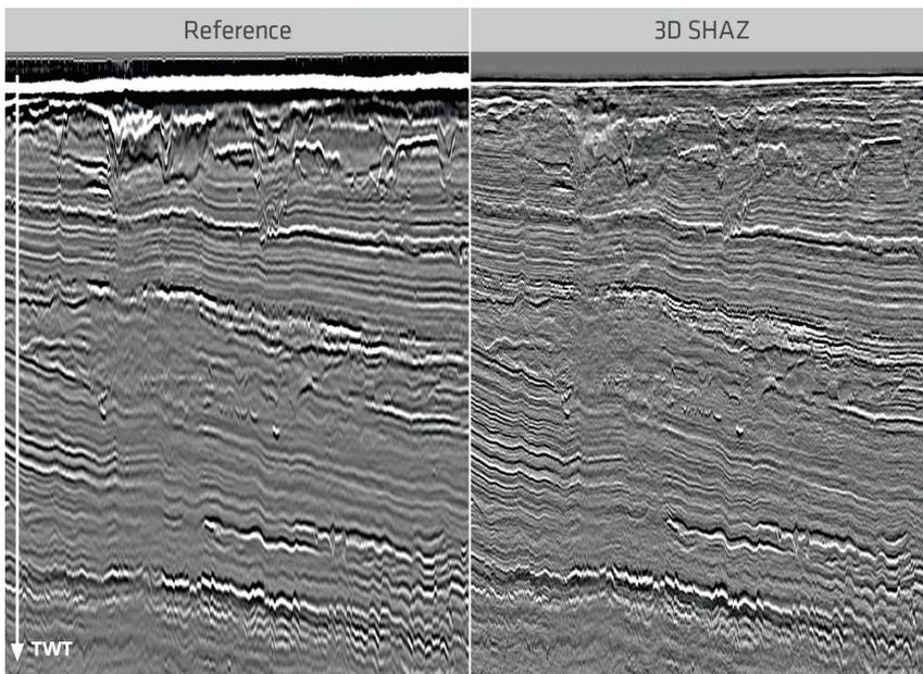
**Figure 5** Crossline (100-1200 ms TWT) sections of the reference cube (left) versus the 3D SHAZ volume (right). White represents an increase in acoustic impedance. A considerable uplift in resolution is shown in the shallowest part of the SHAZ image where SWIM contributes the most. Furthermore, the entire volume benefits from high-resolution 3D imaging.
