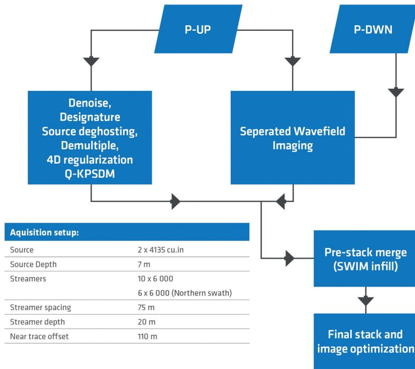
**Figure 3** Survey parameters and 3D SHAZ reprocessing workflow. P-UP and P-DWN are the up-going pressure wavefield and down-going pressure wavefield, respectively.
