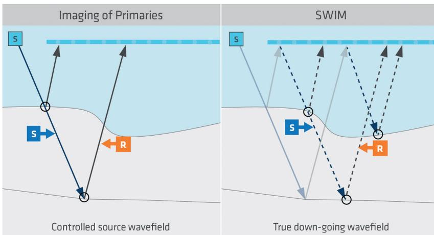
**Figure 4** Illustration of the SWIM imaging principle: conventional primary imaging only (left) against SWIM imaging (right). Note that the main difference comes from the source wavefield (S), which is the recorded down-going wavefield (P-DWN). Its source signature is consistent with the recorded up-going wavefield (P-UP) that is used as the receiver wavefield (R).
