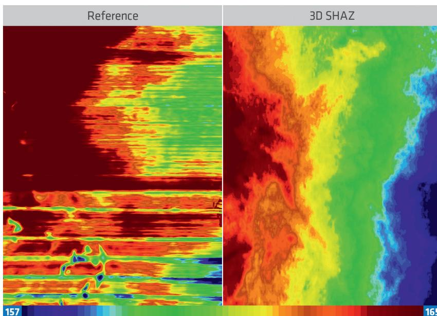
**Figure 7** Isochrone maps (TWT in milliseconds) for the water bottom event derived from the reference 3D seismic data (left) versus the 3D SHAZ data (right). In the reference volume, the southern area that was acquired with a ten-streamer configuration shows stronger acquisition footprint effects. Such effects are not present in the 3D SHAZ volume.
