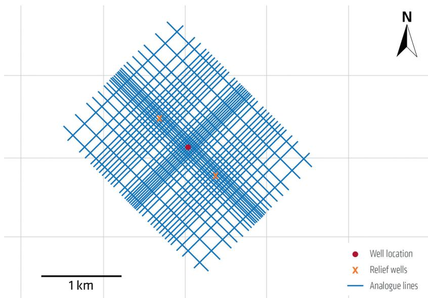
**Figure 1** Typical 2D high-resolution seismic template for a site survey. The line density rapidly decreases with distance from the targeted well location.
