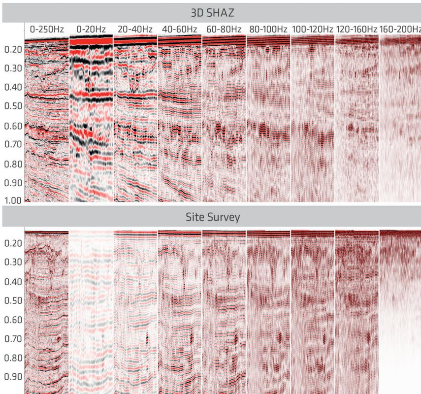
**Figure 8** 3D SHAZ reprocessing frequency panels (top) versus a 2D site survey line (bottom) from an adjacent licence area (TWT in seconds). Red represents an increase in acoustic impedance. The leftmost panel shows the full bandwidth image. The band-limited panels illustrate the signal-to-noise content and event character at various frequency ranges.
