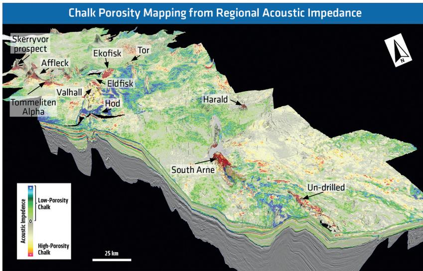
**Figure 6** Regional acoustic impedance amplitude extraction below top chalk horizon from regional dataset (18,000 km<sup>2</sup>). Low acoustic impedance (red) is expected to highlight high-porosity chalk intervals based on findings from the rock physics analysis. High-porosity anomalies correlate very well with chalk fields and highlight some undrilled prospects at this particular stratigraphic interval (e.g. in the south of the dataset).
