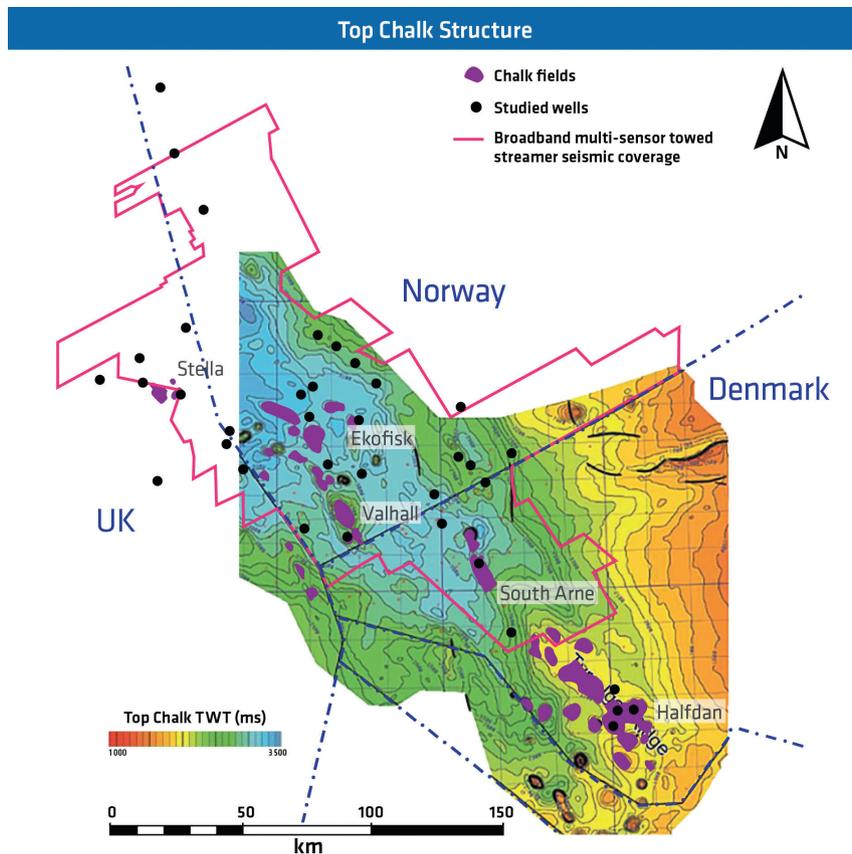
**Figure 3** Base map of the studied area showing top chalk depth variation from north (deeper) to south (shallower). The seismic dataset is outlined in pink, the main chalk fields in purple. The well locations used in the rock physics analysis are shown as black dots (structure map adapted from Mork et al., 2018).
