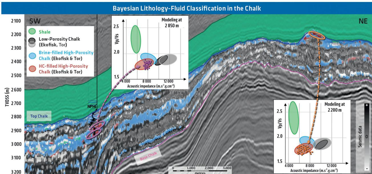
**Figure 8** A promising first-pass porosity and hydrocarbon presence prediction through Bayesian lithology-fluid classification. The various colours correspond to the most likely class from the five lithology-fluid classes established during the depth-dependent rock physics analysis. As part of this Bayesian lithology-fluid classification it is possible to get access to the individual class probability, i.e. probability to be either brine, hydrocarbon-filled or shale or low-porosity chalk.
