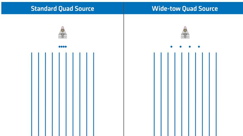
**Figure 1** High-density streamer configurations of 10 streamers at 50 m separation combined with a standard quad-source set-up (left) and a wide-tow quad-source set-up (right). The wide-tow source separation is 62.5 m, resulting in a total source spread with of 187.5 m. The resulting improved near offset separation is shown in Figure 2.
