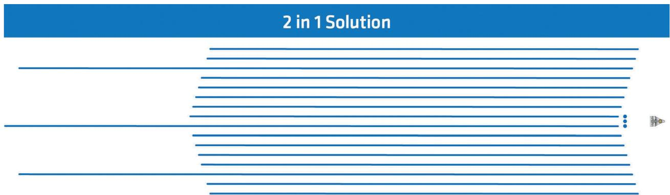
**Figure 7** This '2 in 1 solution' delivers ultra-high density data for imaging and is at the same time a velocity survey: It comprises a high-density 16 x 56.25 m streamer spread with a triple-source set-up. Three out of the 16 streamers were deployed with 10-km long streamer 'tails' providing long offsets for FWI.
