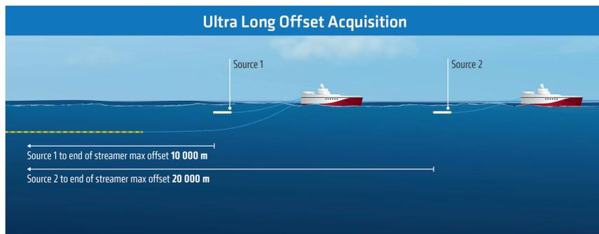
**Figure 6** A two-vessel configuration that can deliver effective source-receiver offsets up to 20 km for FWI applications. The lead vessel only operates sources.
