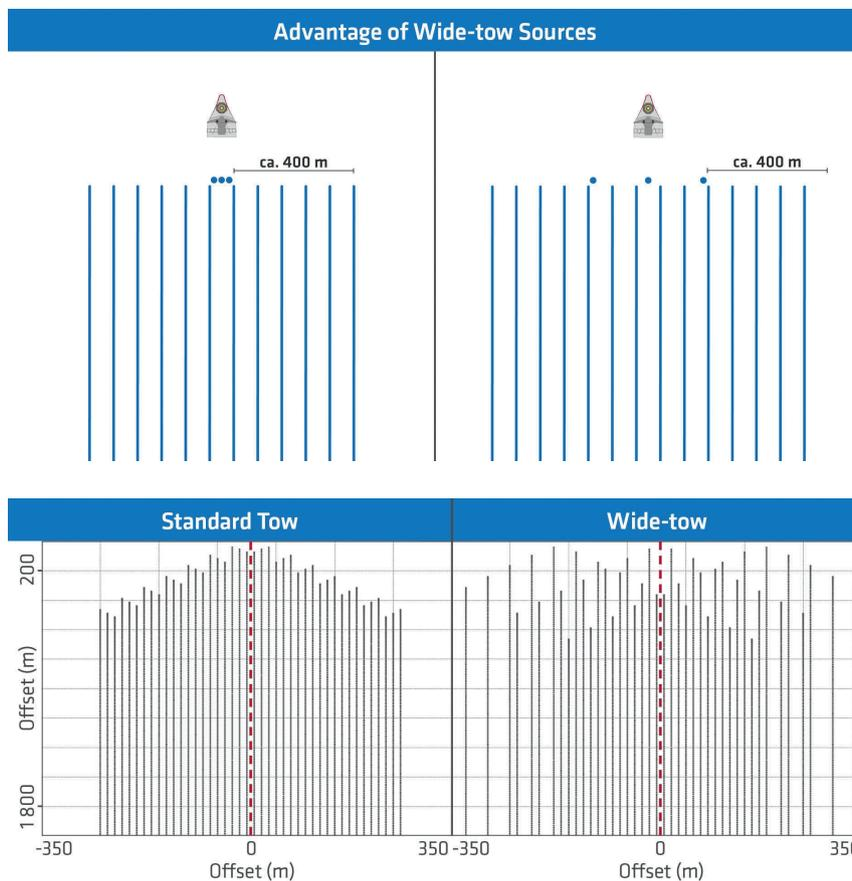
**Figure 3** A 12 x 75 m streamer spread with a standard triple-source configuration (left) and a 14 x 75 m configuration with a wide-tow triple-source (right). The wide-tow configuration provides a smaller distance from source to outer streamer thus increasing efficiency without further compromising the near offsets.
