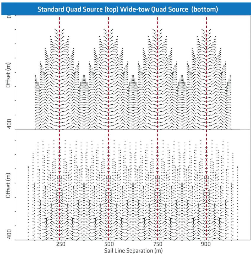
**Figure 2** Near-offset distribution for a quad-source configuration with 12.5 m standard source separation (top) and 62.5 m wide source separation (bottom). The streamer separation is 50 m in both examples. The red dashed lines indicate the centre of each sail line. CMP-X positions are along the x-axis, and source-receiver offsets are along the y-axis. The wide source configuration provides an improved near offset coverage for shallow AVO analysis.
