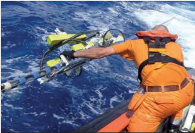
Figure 4 Automated in-sea Streamer Cleaning Units (SCU) have been engineered to allow for continuous proactive barnacle removal during ongoing operation.
