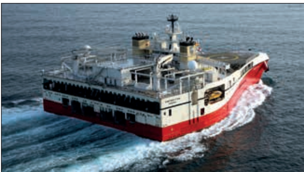
Figure 2 Ramform Atlas photographed while working in the North Sea. The 70 m wide back deck allows safe and efficient deployment and retrieval of a high number of streamers. Note also the calm sea behind the vessel where the two workboats are deployed in cradles.
