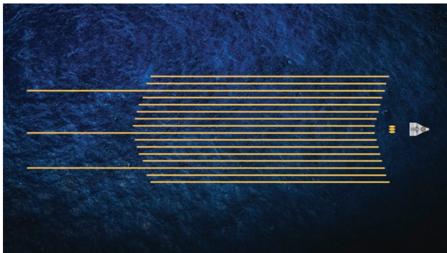
Ultra-dense 16 x 56.25 m streamer spread combined with a triple-source for high-resolution imaging. Three 10 km long long-offset tails were deployed for FWI and imaging of deeper structures.
