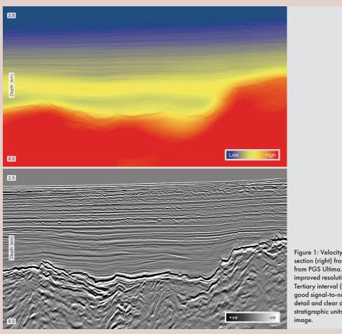
igure 1: Velocity (left) and Reflectivity section (right) from angle gather output from PGS Ultima. The sections show mproved resolution of the velocity in the Tertiary interval (2.5-6 km) and overall good signal-to-noise ratio as well as detail and clear definition of various stratigraphic units in the reflectivity
