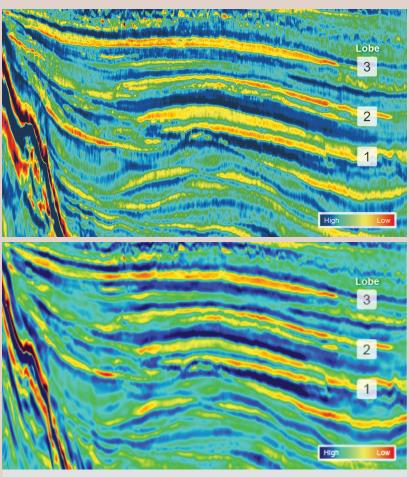
Figure 2: Comparison of relative Vp/Vs from Kirchhoff migration (top) and PGS Ultima (bottom). Note the improved signal-to-noise ratio in the PGS Ultima result. The response of the stacked reservoir units can be seen in both the Kirchhoff migration and the PGS Ultima QI results
