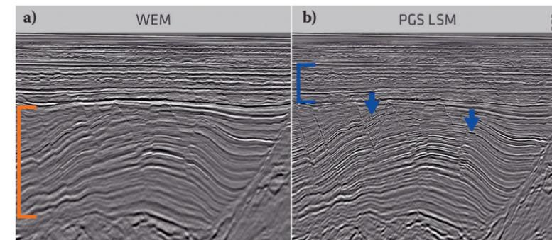
Figure 4: (a) 60 Hz one-way wave equation migration. (b) LSM delivers a higher resolution image with significantly improved fault definition. Blue and orange markers indicate improvements in the Tertiary and Jurassic respectively. Blue arrows indicate improvements in the Cretaceous and Jurassic.
