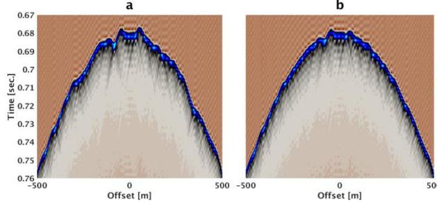
**Figure 1** Sea surface reflectivity shot gather for the very rough sea surface (a) and slightly rough sea surface (b).
