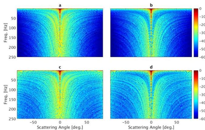
**Figure 2** Plane wave reflection coefficient matrices computed using HKI for the very rough (a) and slightly rough (b) sea surfaces. The plane wave reflection coefficient matrices based on KA for the very rough and slightly rough sea surfaces are shown in (c) and (d), respectively.
