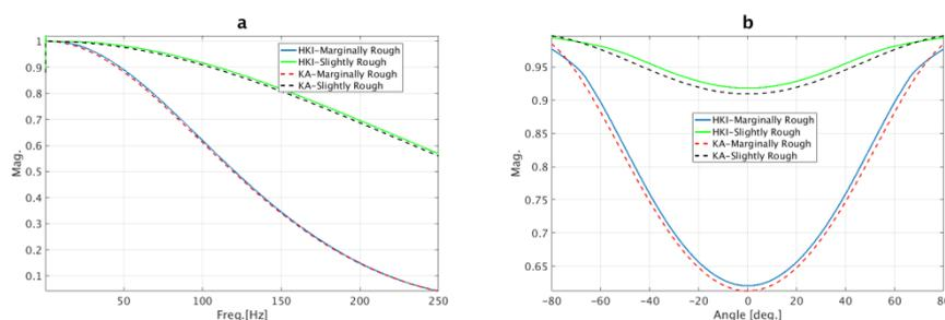
**Figure 3** Specular plane wave reflection coefficient as function of frequency at vertical incidence (a) and angle at 100 Hz (b).
