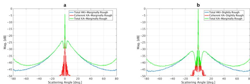
**Figure 4** Total reflection coefficient based on HKI, KA, and coherent KA reflection coefficient for the very rough (a) and slightly rough (b) sea surfaces.
