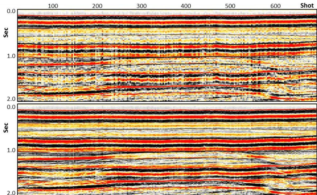
**Figure 3** Ghost-free near offset trace before (upper) and after (lower) signature variation correction.
