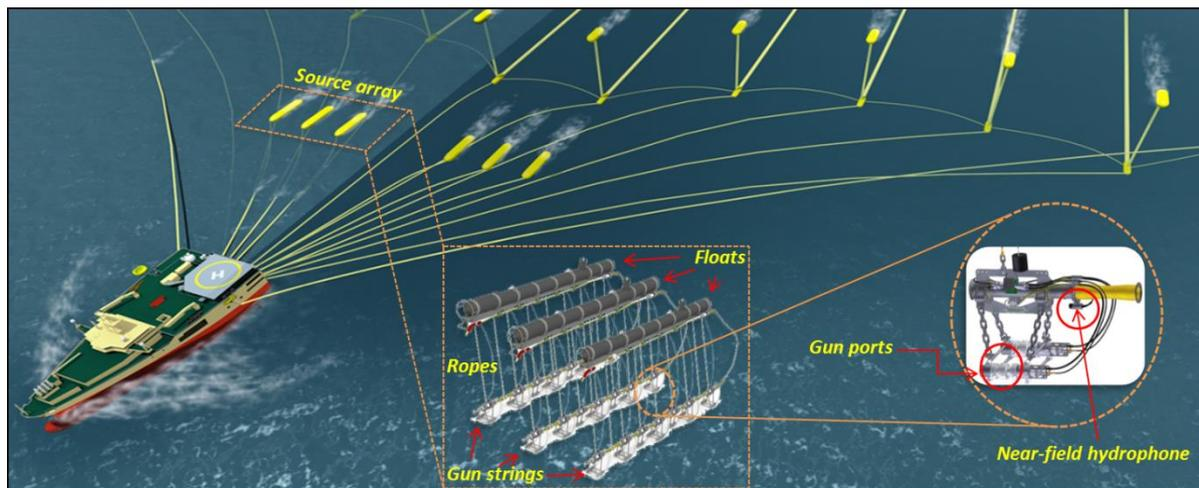
**Figure 1** Dual-source configuration. Each source is made of 3 gun strings suspended below floats.
