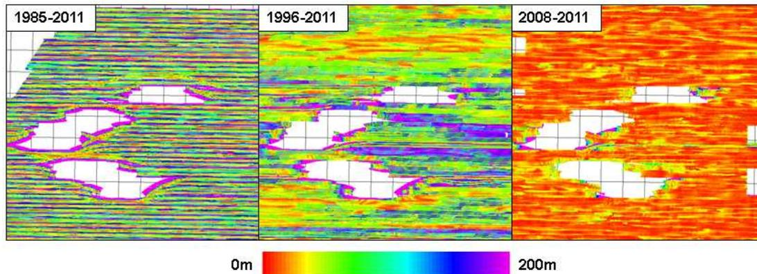
**Figure 1** Maps showing the difference in source and receiver positions between the 2011 vintage and 1985 (left), 1996 (middle) and 2008 (right). The maps clearly show the improvement in acquisition repeatability over the years.
