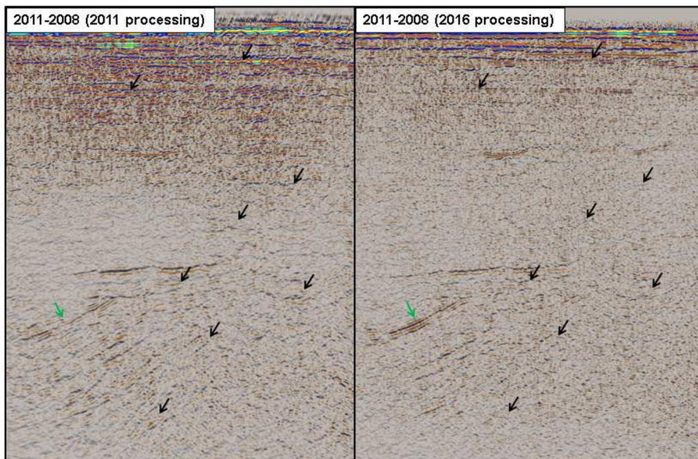
**Figure 3** 4D difference sections between the 2011 and 2008 vintages showing the reduction in 4D noise for data processed in 2016 compared to 2011.
