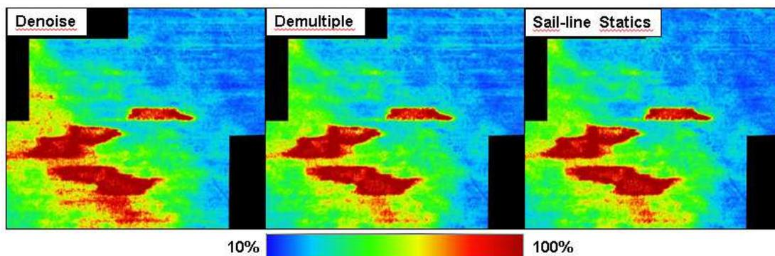
**Figure 2** NRMS maps at the denoise (left), demultiple (middle) and sail-line static corrections (right) stages of the project. Median NRMS values for these maps were 25% for denoise, 24.5% for demultiple and 23.5% for sail-line related statics.
