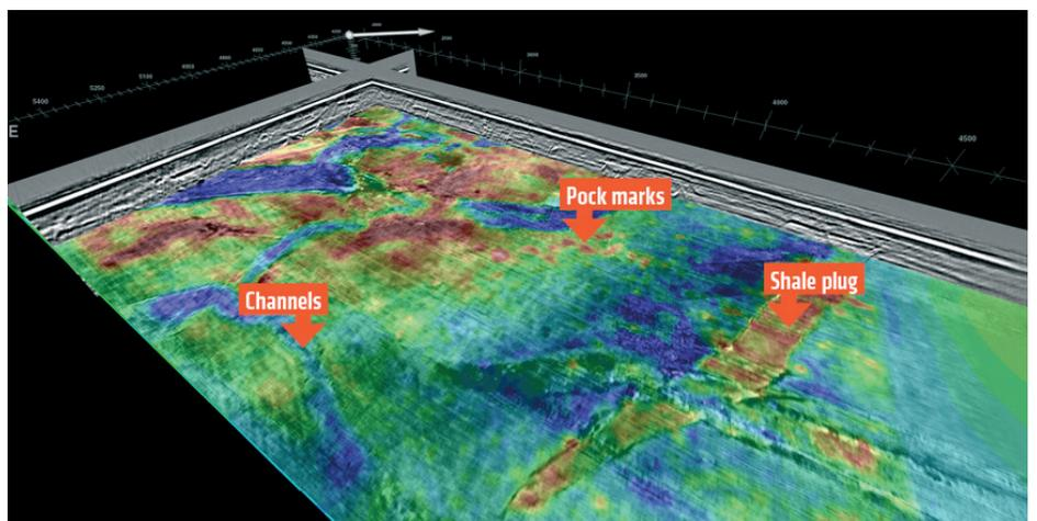
3D View of a depth image at 250 m depth with FWI velocity model overlaid.
