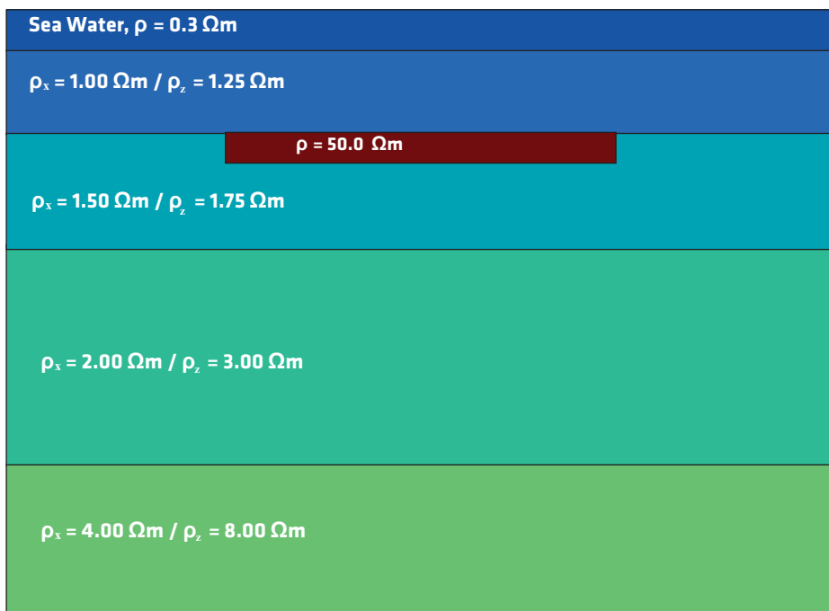
Example of a layered background resistivity model with a resistive anomaly (target) included
